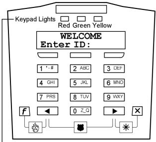
Red Flashing: Protection ON Solid: Partial protection (STAY) Green On Always with power present. Yellow On when trouble condition present. Flashing when there is no AC mains.
