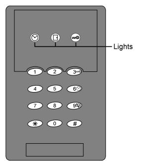
This icon ()) on key 9 is for the command to silence an alarm \* 9 < login>
