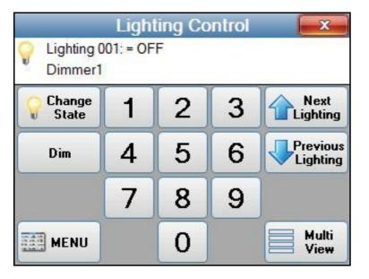
ele In "Single View" mode, the lighting number can be selected with the numeric buttons. Next Lighting and Previous Lighting buttons will move through lighting items that programmed with show enabled.
