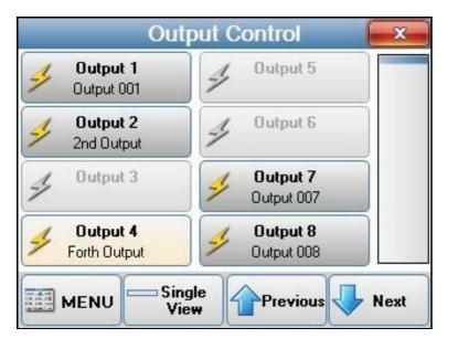
8 output buttons are displayed on the screen at once with each output button displaying the output number and output name.
