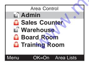
The Area Control screen is now displayed, with the first Area (or Area List) that you are allowed to control highlighted, and a text prompt for the relevant action on that Area, shown at the bottom of the screen. i.e. "OK=On"
