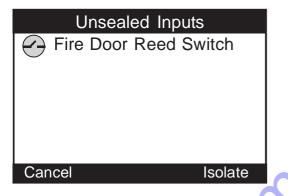
After pressing the <ON> key, the display may show a message like this. It means that any items displayed are either in an alarm state or faulty, and the Area will not turn ON.
