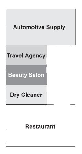
areas, portions of the building can be independently armed and disarmed. In the case of the first building illustrated, an employee can work in the repair shop while the showroom, offices, and warehouse are armed. Similarly, in the case of the second illustration, the restaurant can remain open after the other shops are closed and armed.
